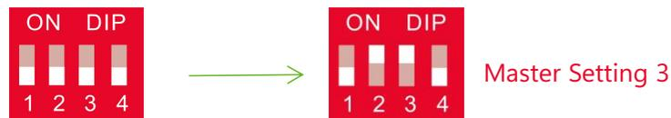
5. If the battery communicates with the Schneider Context Series, turn the master DIP switch "#1" and "#3" to "ON".
