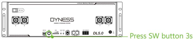
3. Check the system output voltage and led status
