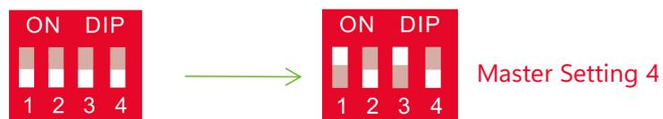
6. When you setup the master DIP as setting 1~4, all the slaves keep the DIP 0000, no need to change.
